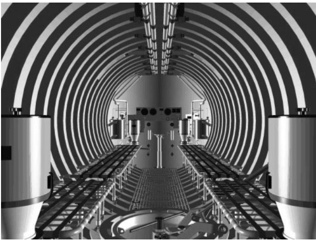
Figure 7: Internal View of PRM Rescue Chamber (looking aft)
